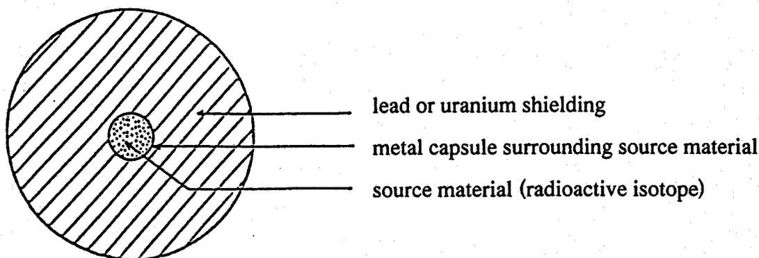
**FIGURE 1: CONSTRUCTION OF A TYPICAL SEALED SOURCE**
