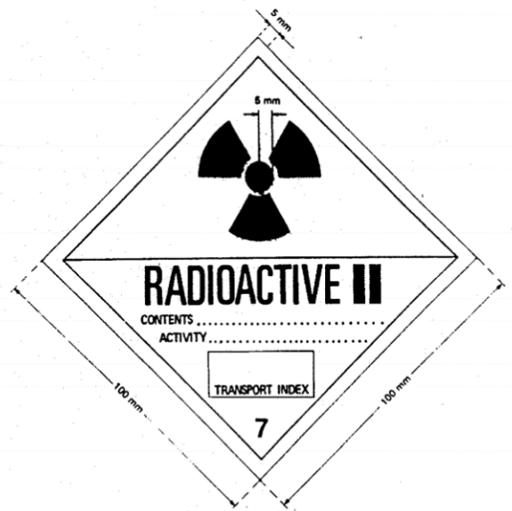
Fig 3: Category II-YELLOW label. The background colour of the upper half of the label shall be yellow and of the lower half white, the colour of the trefoil and the printing shall be black, and the colour of the category bars shall be red.
